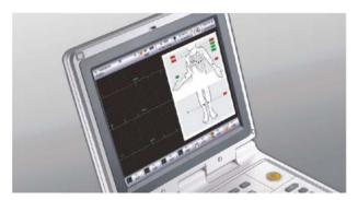
Lead Status Diagram to show ECG leads conductivity
